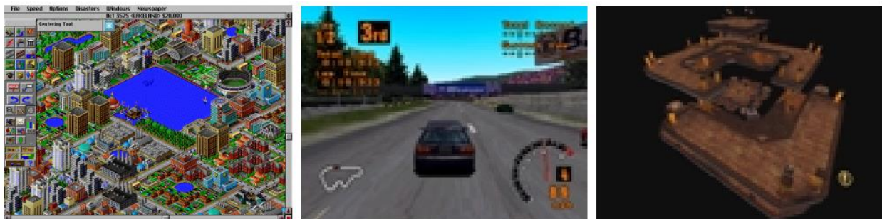
Figure 5: (a) isometric projection, (b) central perspective with one, (c) perspective with three vanishing points
