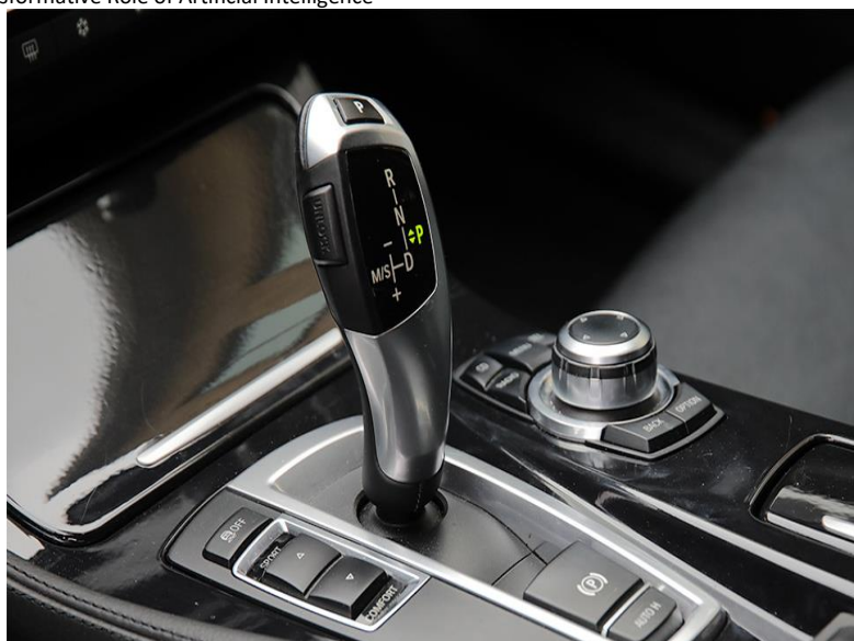
Fig. 2.4 Automatic Car Gear Shifter. (Esquire, 2020)
