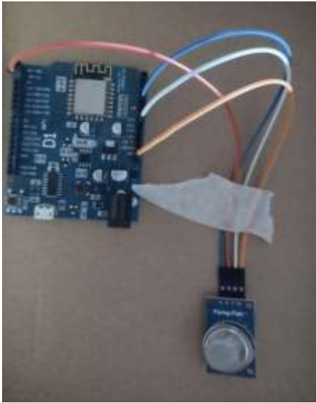
Figure 4. MQ135 Gas sensor linked to ESP8266 Microcontroller.
