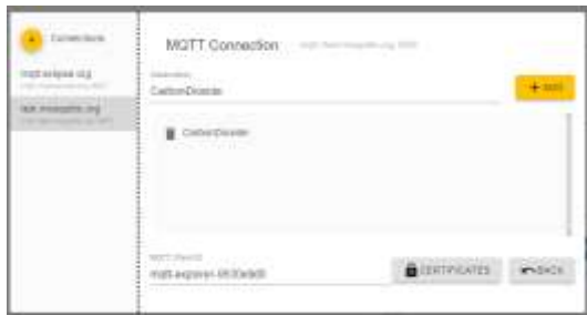
Figure 11. A simple subscription to the topic CarbonDioxide using MQTT-explorer.
