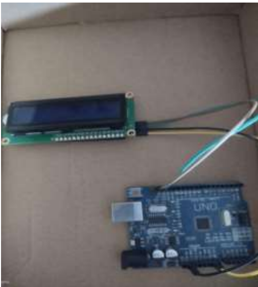
Figure 5. LCD Display linked to ARDUINO UNO Microcontroller.
