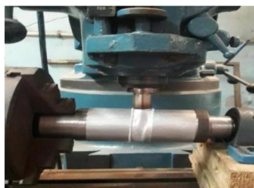
Figure 1 FSW in milling machine
