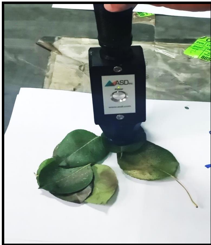
Fig.4.Measuring the reflectivity of plant before burial(20/9/2021).
