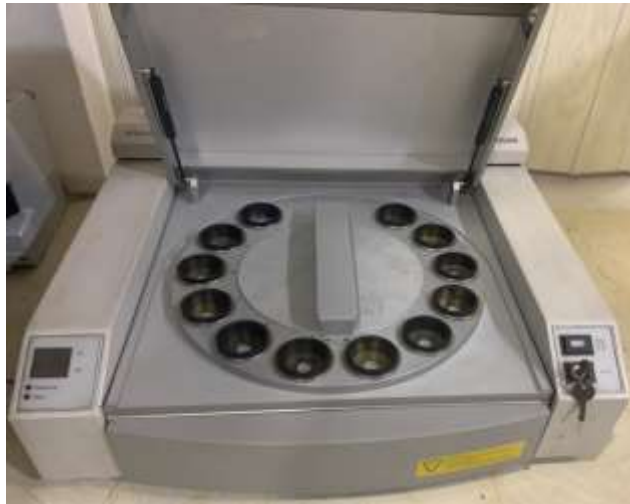
Figure.1: shows the XRF- Minipal2 instrument.
