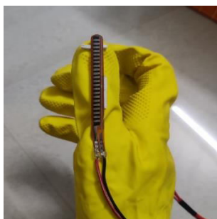
Fig 8. Flex sensor embedded in the glove
