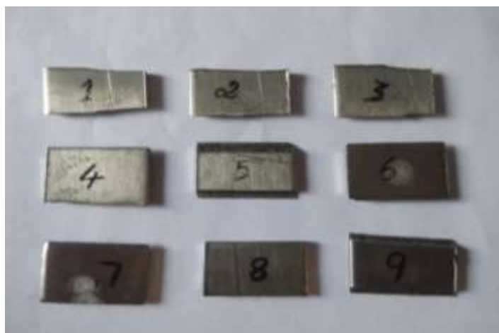
Fig 4: Monel 400 after Machining
