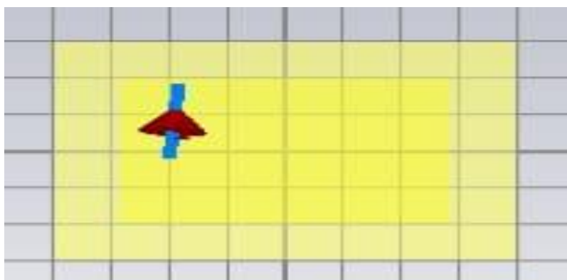
Fig 5.1 Design of patch without defective ground
