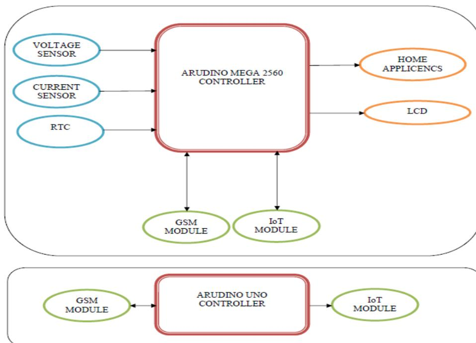
Figure 1: Architecture of Intelligent Controller and Base Station.
