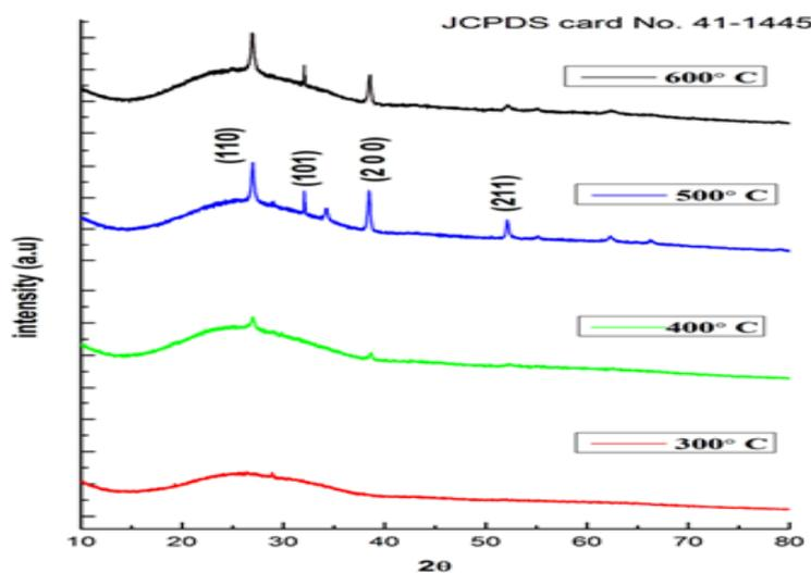
Figure 4. X-Ray Diffraction spectra of SnO<sub>2</sub> thin films deposited at various temperatures.
