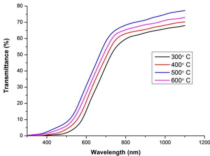
**Figure 5. Transmittance spectra of SnO<sub>2</sub> thin films.**
