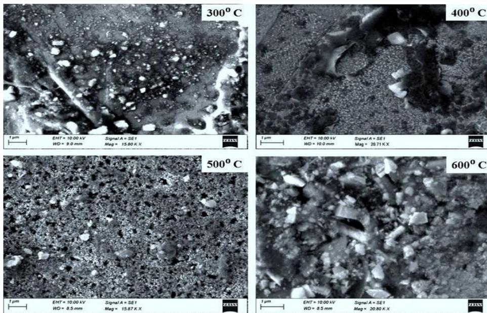
Figure 3. SEM images of SnO<sub>2</sub> thin films for different substrate temperatures.
