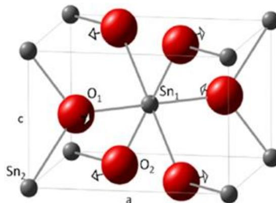
Figure 1. The rutile structure of SnO<sub>2</sub>[32].
