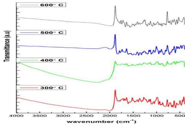
Figure 8. FTIR spectra of SnO<sub>2</sub> thin films.
