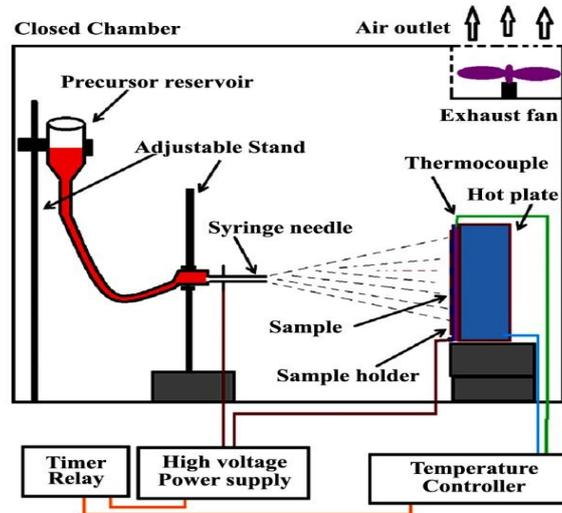
Figure 2. Schematic diagram of the Homemade spray pyrolysis setup.
