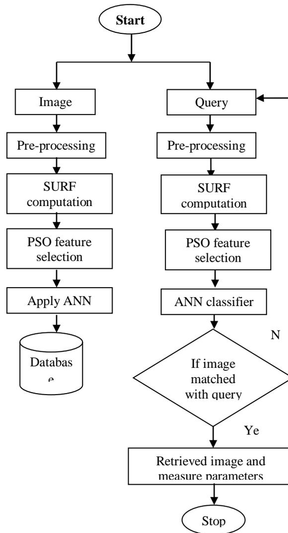
**Fig. 1 Flow of Proposed CBIR based satellite image retrieval system**
