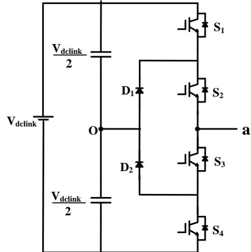
Fig.2. single phase 3 level Diode clamp MLI
