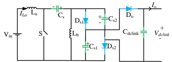
Figure.1 Modified sepic converter
