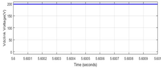
Figure.6. Vdc link voltage of dc converter with change in the reference value
