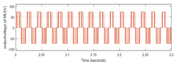
Figure.5. Single phase output voltage of MLI
