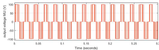
Figure.7. Single phase output voltage of a MLI
