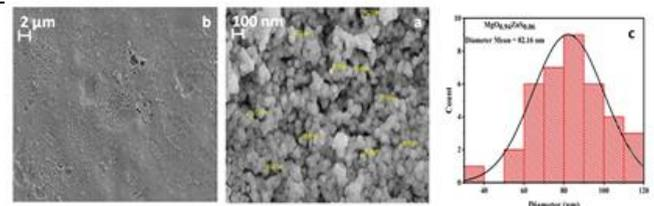
**Figure 5.** (a,b) (FE-SEM) images, (c) grain size distribution diagram of the thin film (MgO<sub>0.94</sub>ZnS<sub>0.06</sub>).
