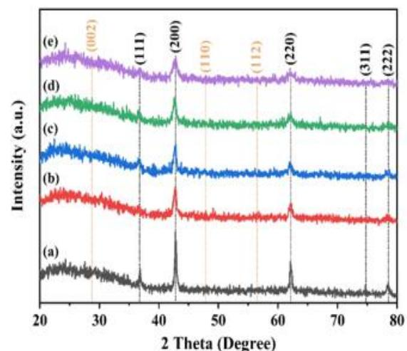
**Figure 1.** X-ray diffraction patterns of thin films (MgO) doped with zinc sulfide (ZnS): (a) (MgO) pure, (b) 2% (ZnS), (c) 4% (ZnS), (d) 6% (ZnS), (e) 8% (ZnS)
