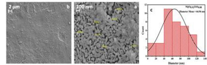
**Figure 6.** (a,b) (FE-SEM) images, (c) grain size distribution diagram of the thin film (MgO<sub>0.92</sub>ZnS<sub>0.08</sub>).
