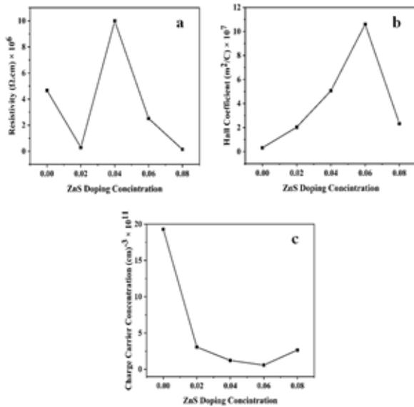
Figure 7. shows the values of (a) resistivity, (b) Hall coefficient, and (c) concentration of charge carriers, as a function of doping ratios for all prepared films.
