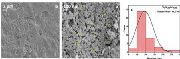
**Figure 4.** (a,b) (FE-SEM) images, (c) grain size distribution diagram of the thin film (MgO<sub>0.96</sub>ZnS<sub>0.04</sub>).
