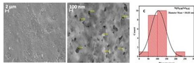
**Figure 3.** (a,b) (FE-SEM) images, (c) grain size distribution diagram of the thin film (MgO<sub>0.98</sub>ZnS<sub>0.02</sub>).
