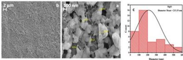
**Figure 2.** (a,b) (FE-SEM) images, (c) grain size distribution diagram of the thin film (MgO).
