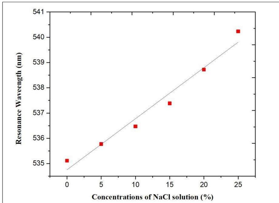
**Figure 4: Resonance wavelength shift vs concentration of NaCl solution**
