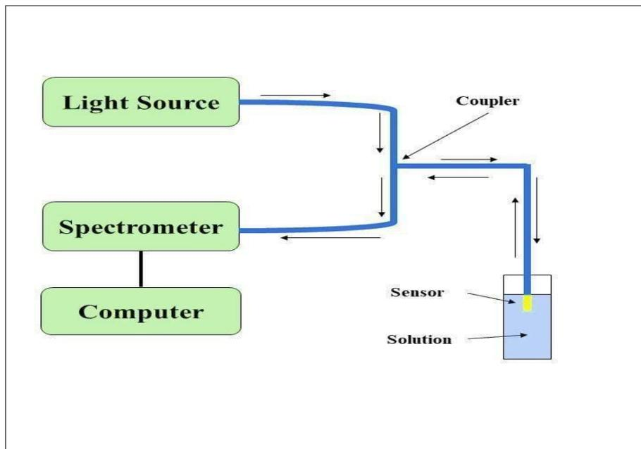
Figure 2: "Schematic diagram of the experiment system".
