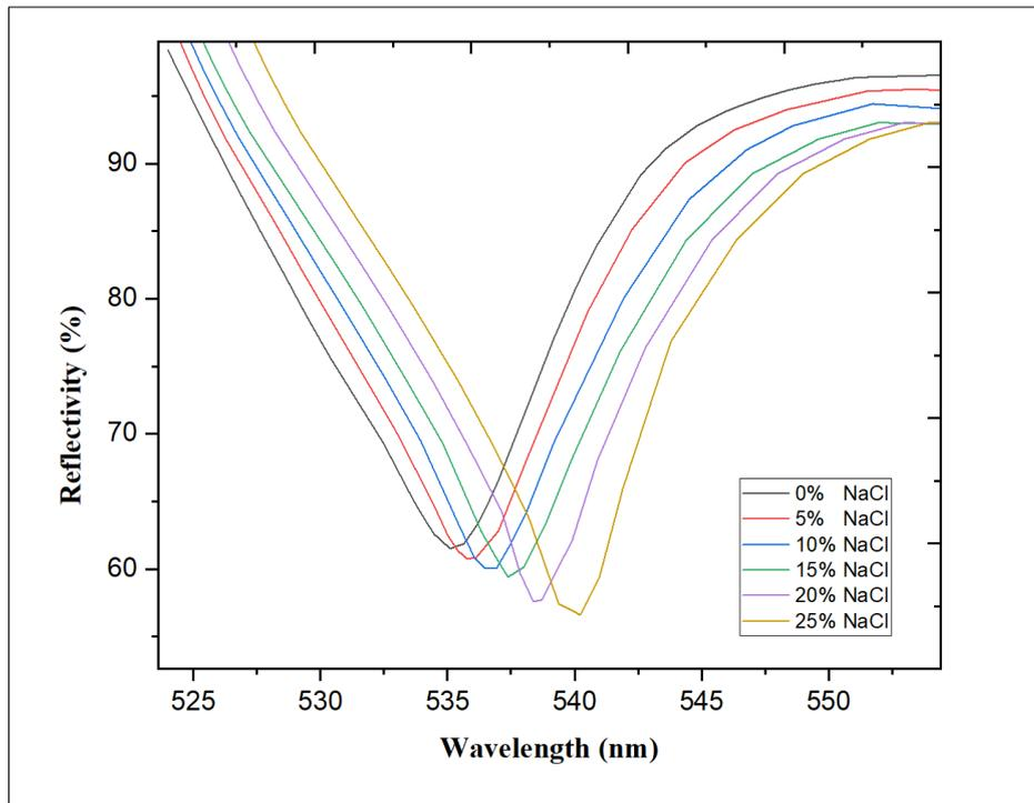
**Figure 3: SPR reflection range of various concentrations of NaCl solution.**
