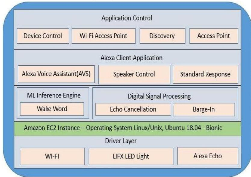
**Figure 2:** Block diagram for smart lighting system.
