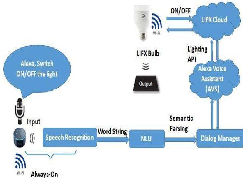
**Figure 1:** Architecture for voice-based smart lighting system
