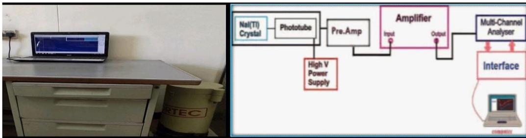
**Figure 2.** The diagram of the NaI(Tl) detector
