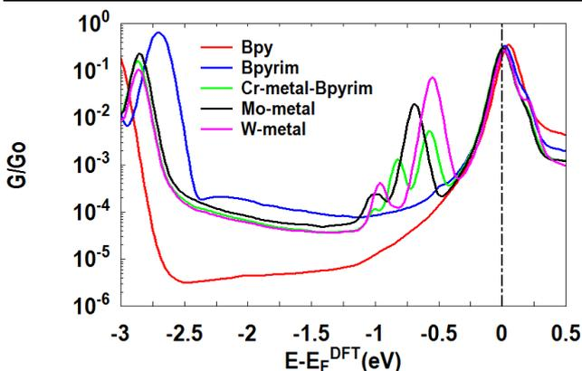
**Figure 4.** Electrical conductance values at room temperature as a function of energy for Bpy (red), Bpyrim (blue), Cr-metal (green), Mo-metal (black), and W-metal (pink)
