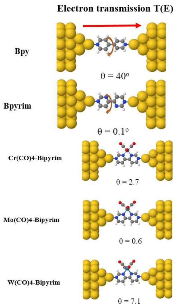
**Figure 1.** Molecular structures of a set of Bpy, Bpyrim, and  $X(\text{CO})_4$ -Bipyrimidine molecules between two gold leads at different metal centre (Cr, Mo, W) complexes
