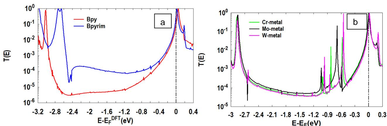
**Figure 3.** Theoretical calculation of transport coefficient as a function of the Fermi energy for a) Bpy and Bpyrimidine b) X(CO)<sub>4</sub>-bipyrimidine molecular junctions
