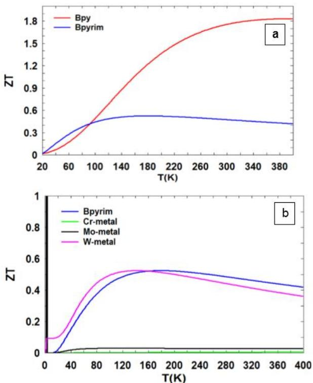
**Figure 7.** The electronic contribution to the figure of merit  $ZT_e$  at Fermi energy as a function of room temperature for a) Bpy and Bpyrim b) central atom (Cr, Mo, and W) metal complexes
