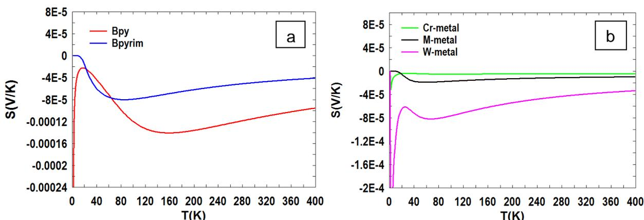
**Figure 5.** Seebeck coefficient  $S$  as a function of the temperature for a) Bpy and Bpyrim b) X(CO)<sub>4</sub>-bipyrimidine molecular junctions at Fermi energy
