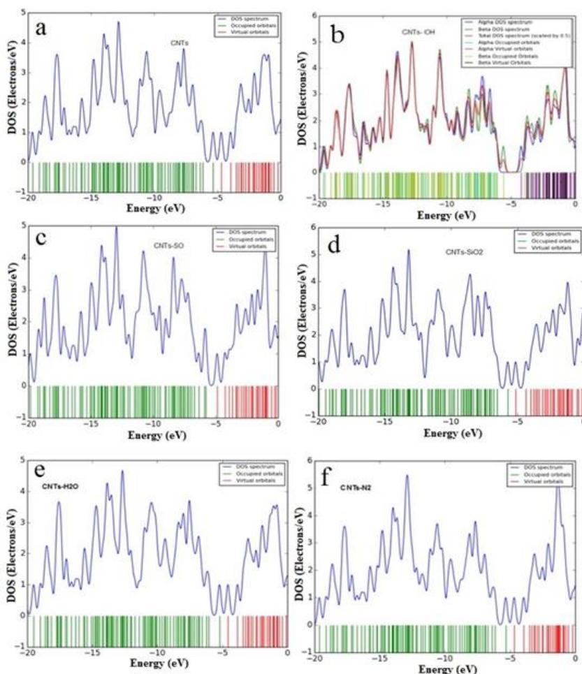
**Fig. 2.** The States of Density for the structure for (a) CNTs, (b) CNTs-OH, (c) CNTs-SO, (d) CNTs-SiO<sub>2</sub>, (e) CNTs-H<sub>2</sub>O and (f) CNTs-N<sub>2</sub> structures for energy
