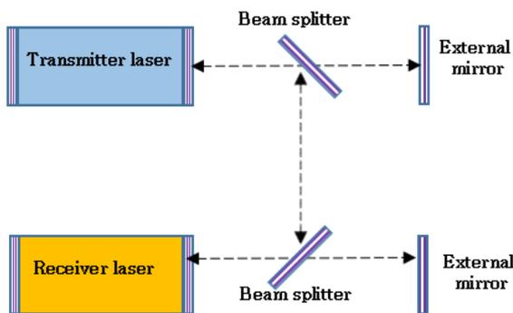
**Figure 1.** Mutual coupling regime (transmitter laser and receiver lasers)
