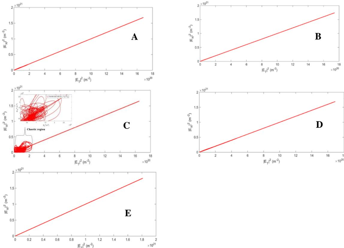
Figure 3. Photon density correlation plot between transmitter laser and receiver lasers at (a)  $\alpha = 2$ , (b)  $\alpha = 2.5$ , (c)  $\alpha = 3$ , (d)  $\alpha = 3.5$  and (e)  $\alpha = 4$
