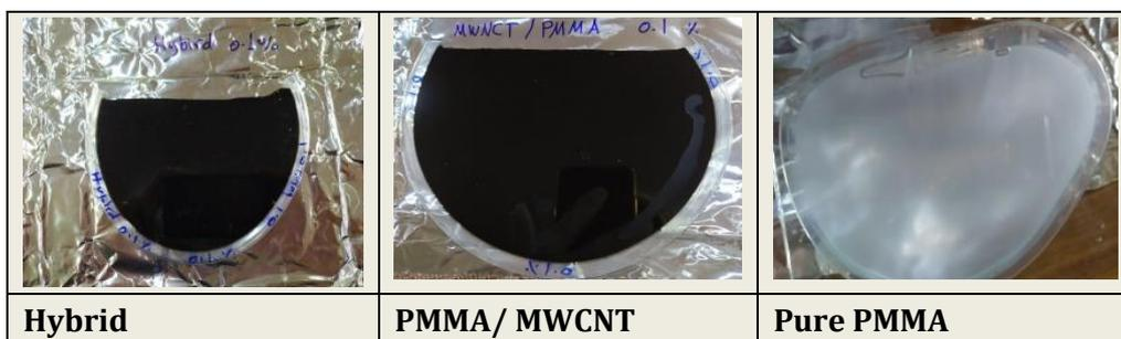
**Figure 1.** Samples produced by in-situ polymerization
