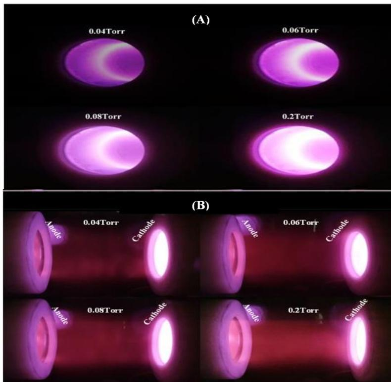
Figure 2. The influence of gas pressure on the normal glow discharge regions, in two groups: A) Internal cathode cavity and B) Inter-electrodes gap.
