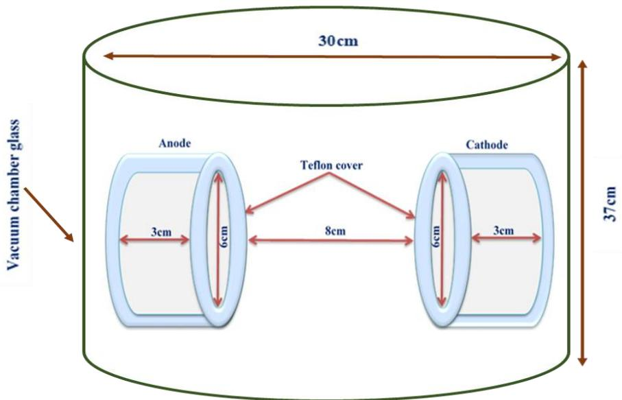
Figure 1. Schematic of the hollow electrodes discharge chamber
