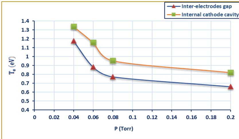
Figure 7. The variation of  $T_e$  against the gas pressure in two regions: inter-electrodes gap and internal cathode cavity
