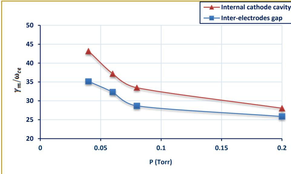
Figure 11. The growth rate as a function of gas pressure
