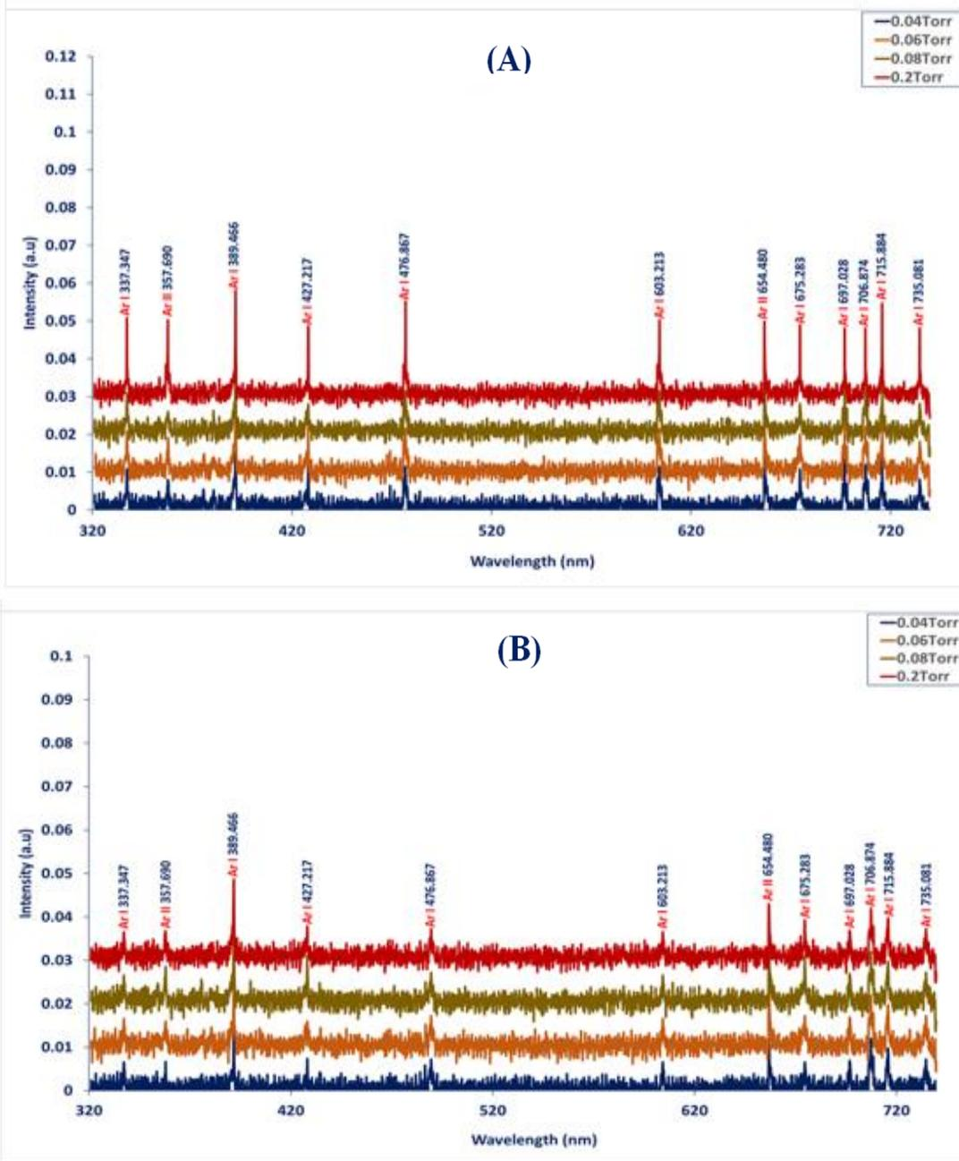
**Figure 4.** The optical emission spectra of Ar plasma at different gas pressures, in two regions: A) internal cathode cavity and B) inter-electrodes gap, in the magnetic mirror
