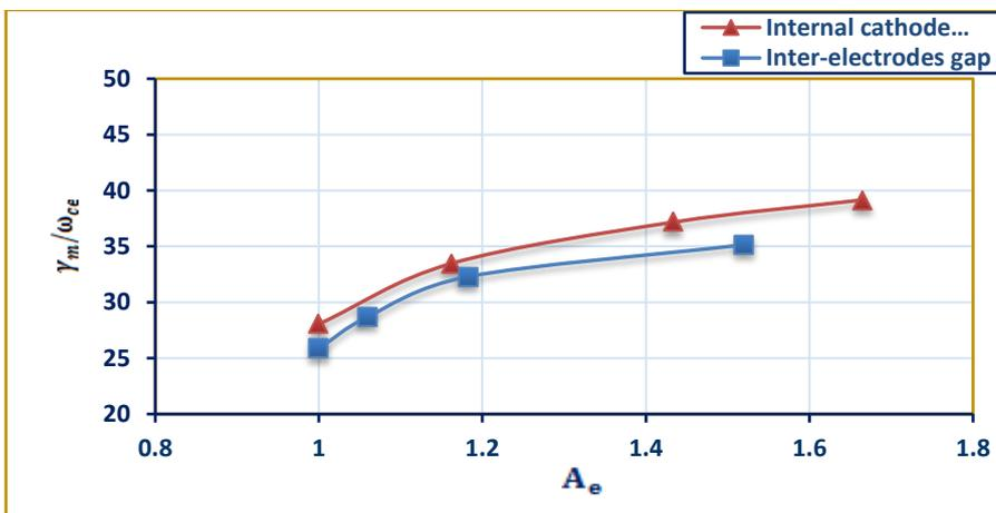
Figure 10. The growth rate as a function of electron temperature anisotropy
