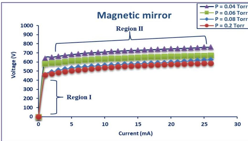
Figure 3. I-V curves of Argon gas for HED, with magnetic mirror.
