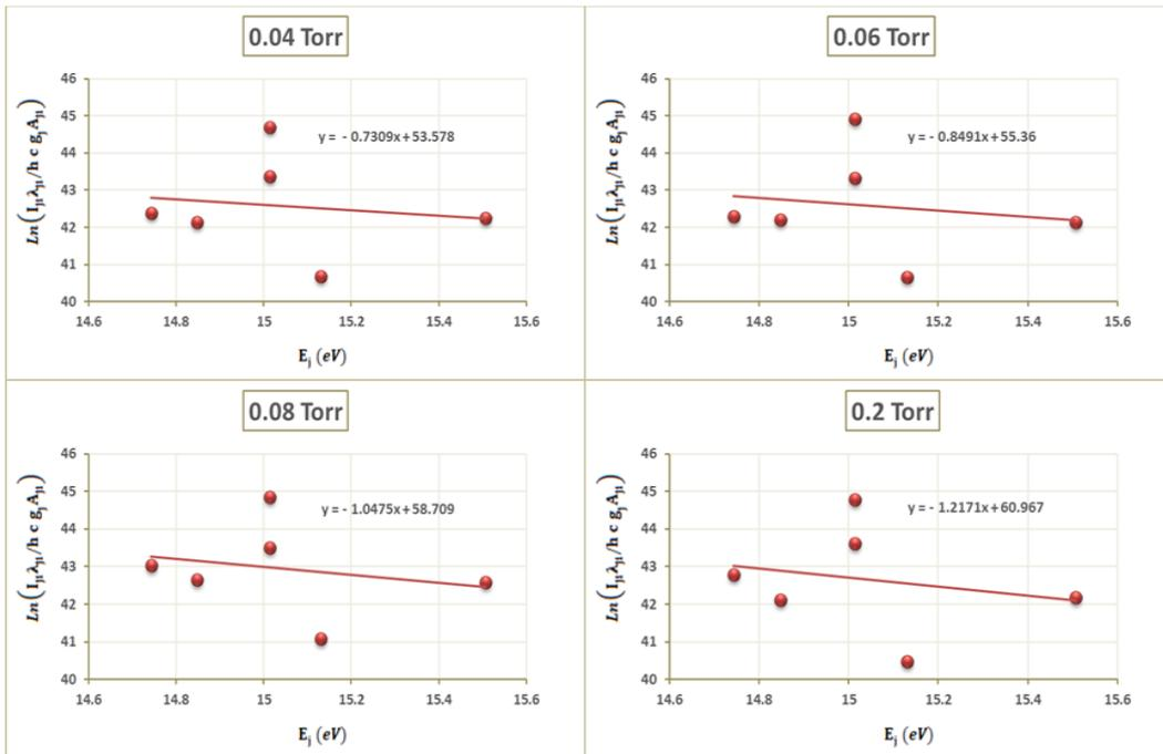
Figure 6. Boltzmann plot for ArI peaks using the hollow electrodes system at different gas pressures, in the internal cathode cavity
