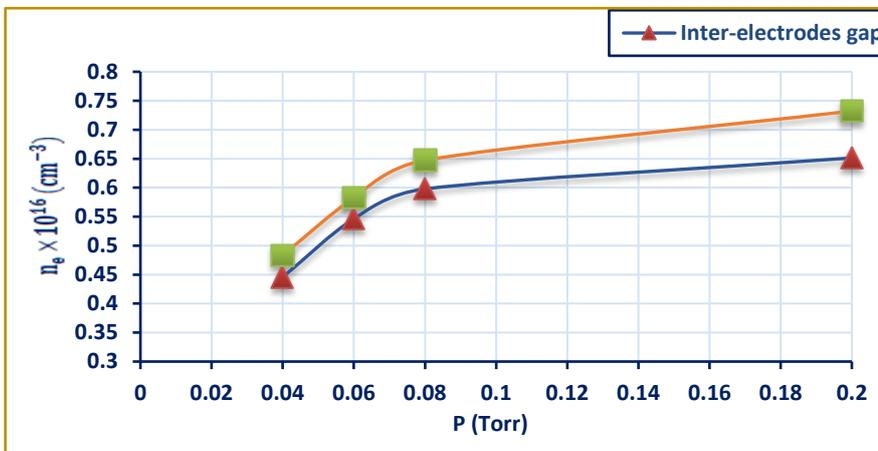
Figure 8. The difference of  $n_e$  against the gas pressure in two regions: inter-electrodes gap and internal cathode cavity
