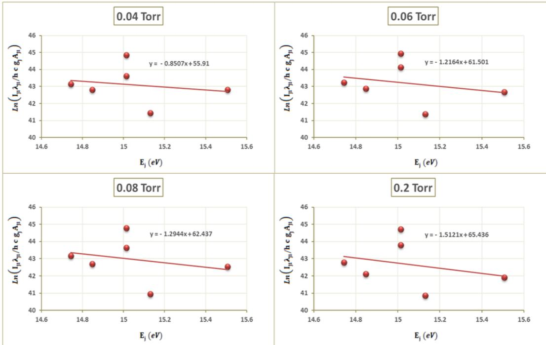
Figure 5. Boltzmann plot for ArI peaks using the hollow electrodes system at different gas pressures, in the inter-electrodes gap
