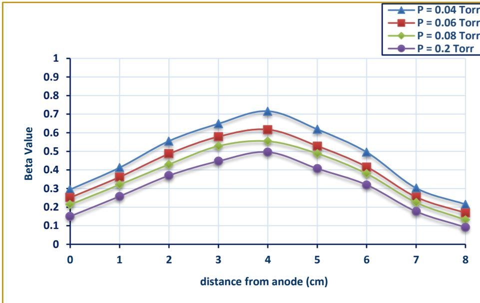
Figure 9. The variation of  $\beta$ -value with the distance from anode for the inter-electrodes gap at different gas pressures
