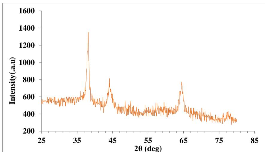
Fig. 2. XRD patterns for Nanoparticle gold thin films
