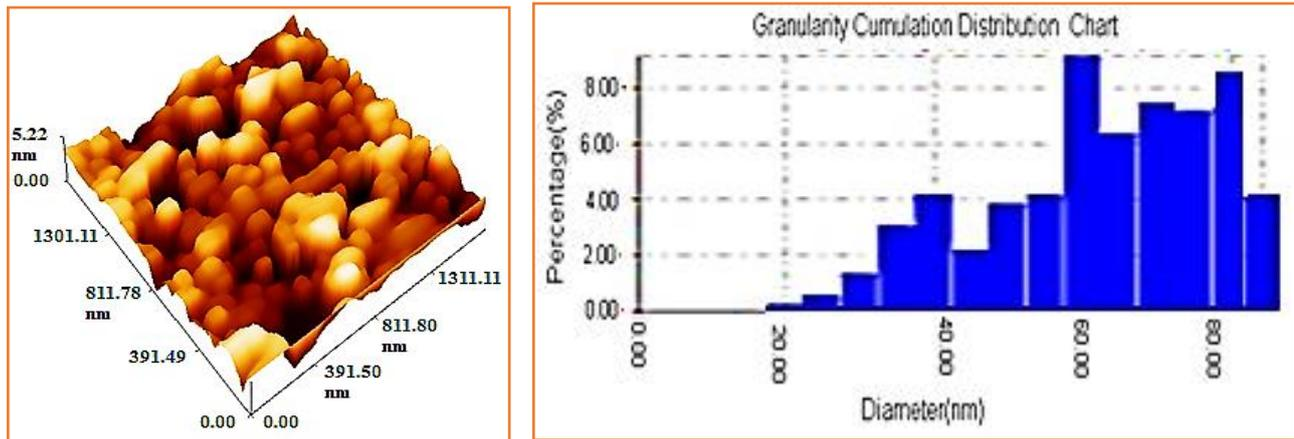
Fig. 3. 3-D AFM photos and chart of the nano-granola
