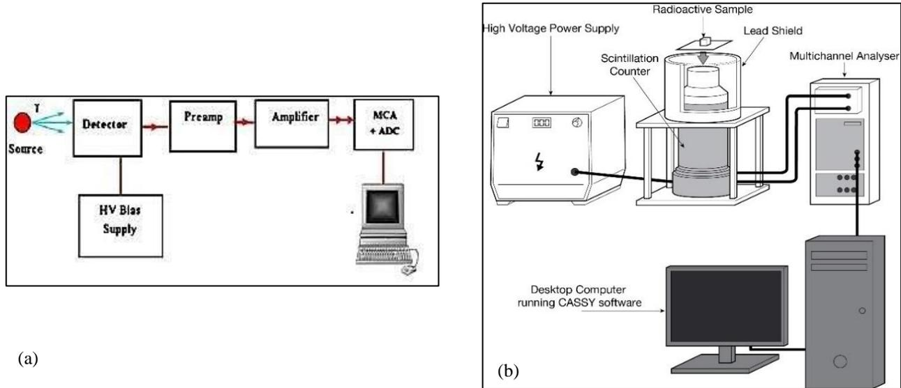
Figure 1. (a) low level background gamma-ray-spectrometer diagram (b) Scintillation counter as a spectrometer (Hadi et al., 2021).
