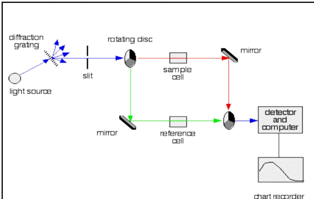
**Figure 16.** Illustration of the components of the dual beam spectrometer (Skoog et al., 2007)
