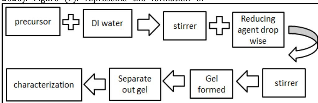
Figure 8. Represents the formation of nanomaterials by the sol-gel method (Iqbal et al., 2017)
