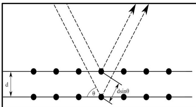
Figure 11. Crystalline levels and Braque's law (Yamaguchi et al., 2007)
