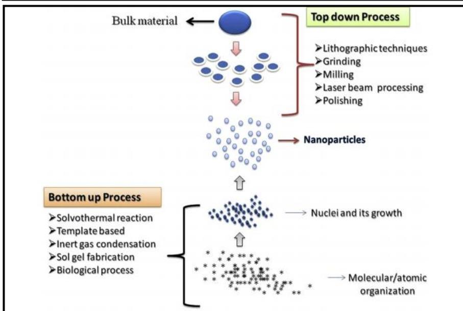
Figure 4. Represents the techniques for obtaining nanomaterials (Baker et al., 2013)
