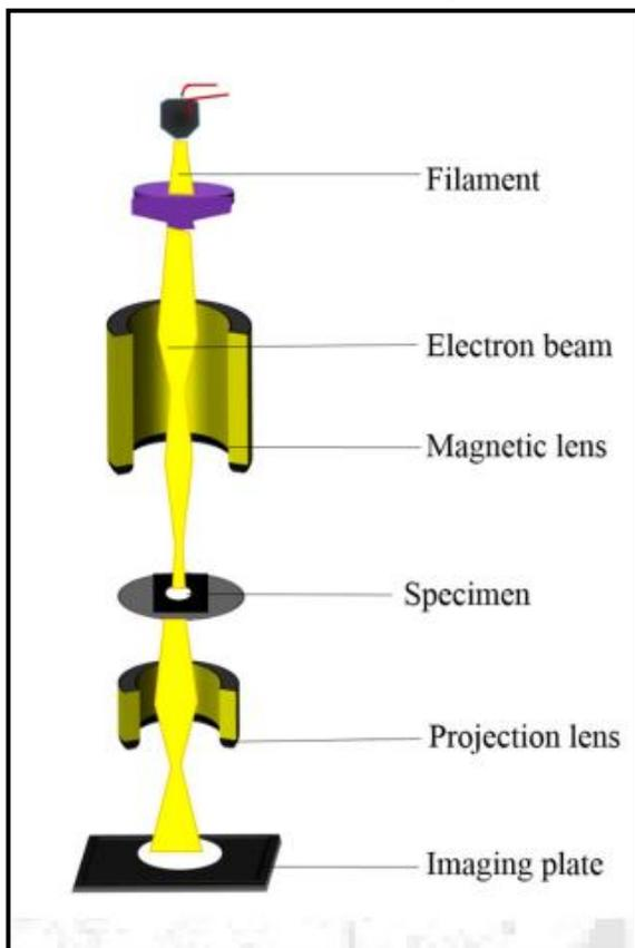
Figure 13. Represents the transmission electron microscope (McDonagh, 2015)
