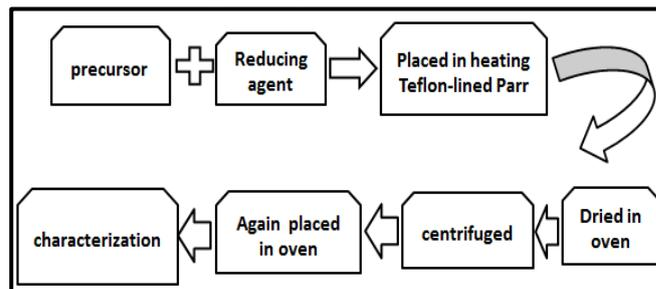
Figure 7. Represents the formation of nanomaterials by the hydrothermal method (Iqbal et al., 2017)
