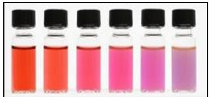
Figure 2. Shows the change in the color of gold according to the size of its grains (Aldrich, 2015).
