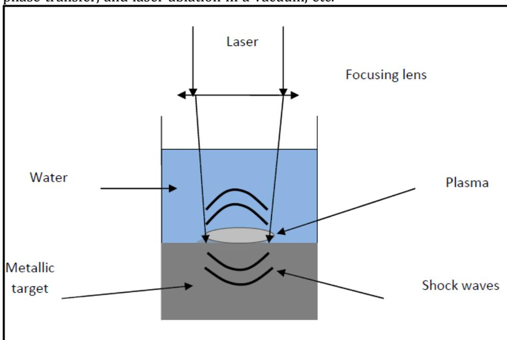
Figure 10. Represents the formation of nanomaterials by the method of laser ablation in a liquid (Zhu et al., 2001).
