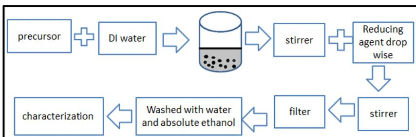
Figure 5. Represents the method of sedimentation to form the nanomaterial (Iqbal et al., 2017).
