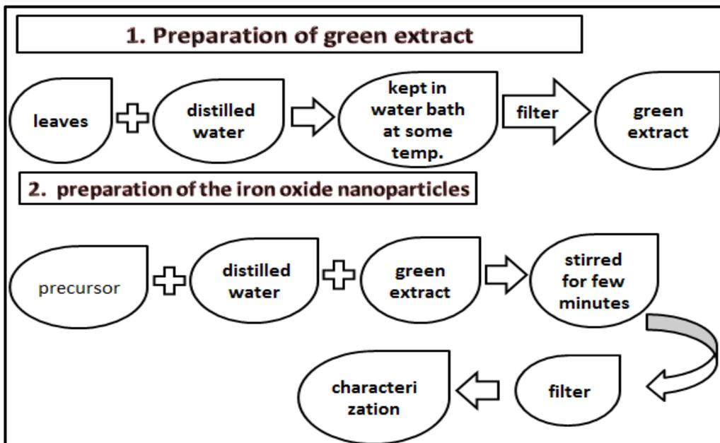
Figure 9. Represents the formation of nanomaterials by the green synthesis method (Iqbal et al., 2017)
