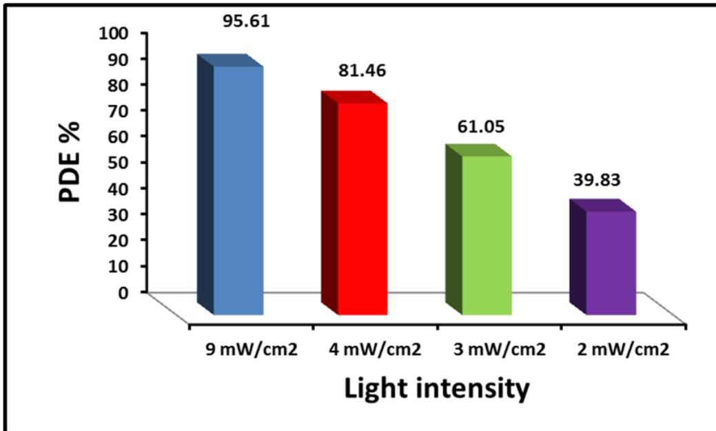
Fig. 6. Photocatalytic degradation efficiency using 0.2g / 100 ml ZnO / V<sub>2</sub>O<sub>5</sub> nanocomposite and 20 ppm of safranin-T dye
