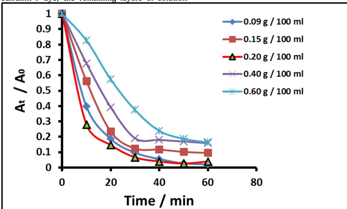
Fig. 3. Variation in ( $A_t/A_0$ ) with time of irradiation at 20 ppm of the prepared dye
