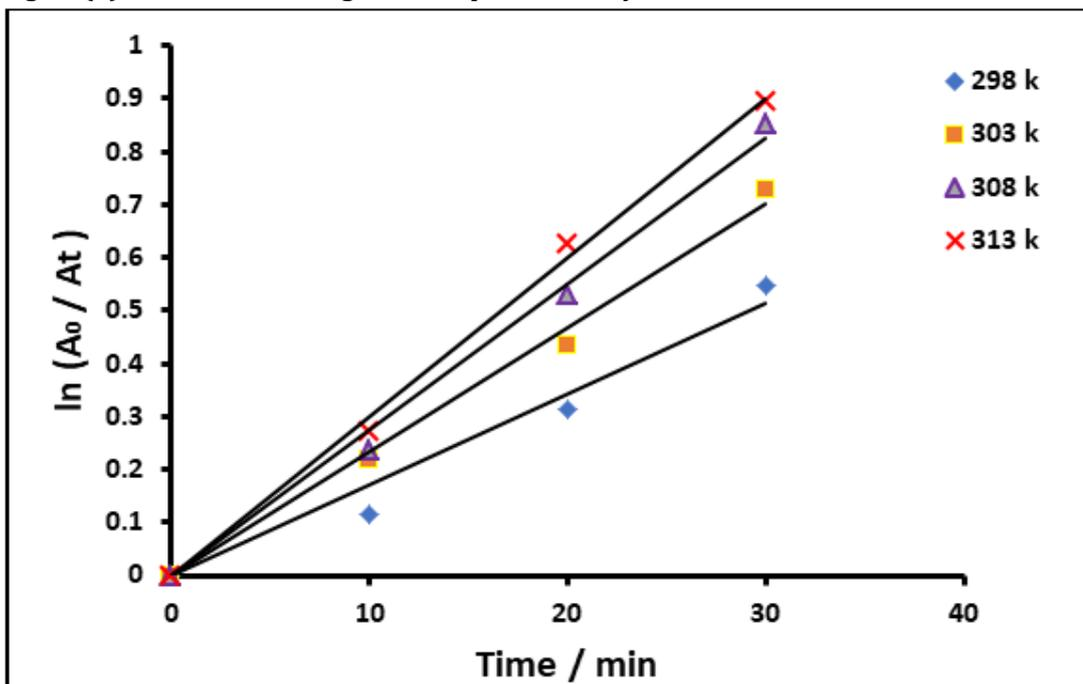
Figure 7. Change of “ln (A<sub>0</sub> / A<sub>t</sub>)” with time of irradiation at different temperature using UV radiation, initial Safranin-T dye concentrations = 20 ppm, amount of photo catalyst = 0.20 g / 100 cm<sup>3</sup>
