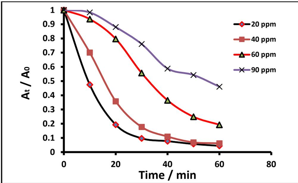
Fig. 4. Variation in (A<sub>t</sub>/A<sub>0</sub>) with time of irradiation at different concentrations of dye
