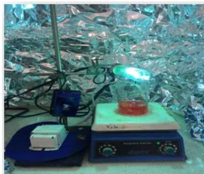
Fig. 2. Main parts of the photocatalytic-cell used in Photocatalytic-degradation of Safranin-T dye
