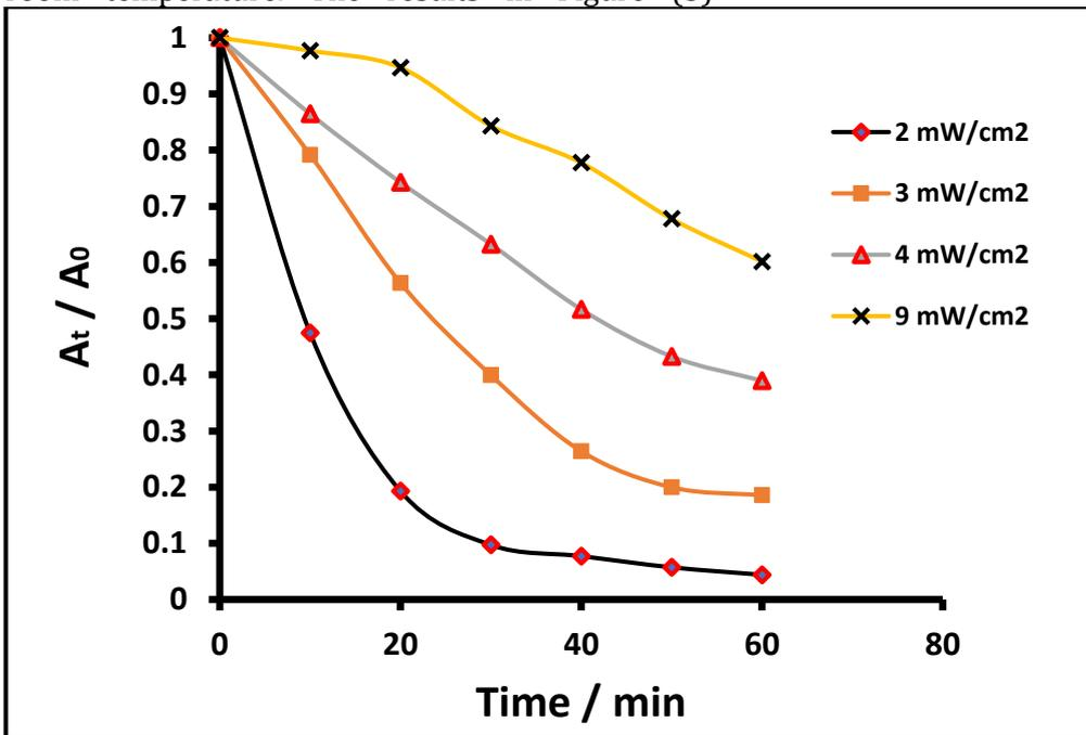
Fig. 5. Variation in (A<sub>t</sub>/A<sub>0</sub>) with irradiation time at different light intensity
