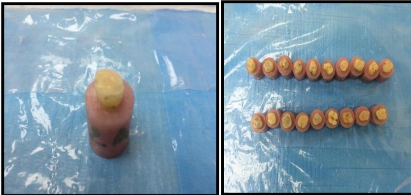
Figure 1. Extracted tooth specimen mounted in acrylic base.
