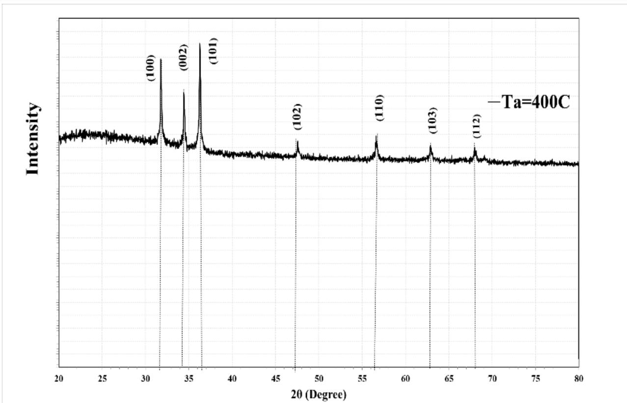
**Figure 2.** X-ray diffraction diagram of the annealed ZnO membrane at 400oC
