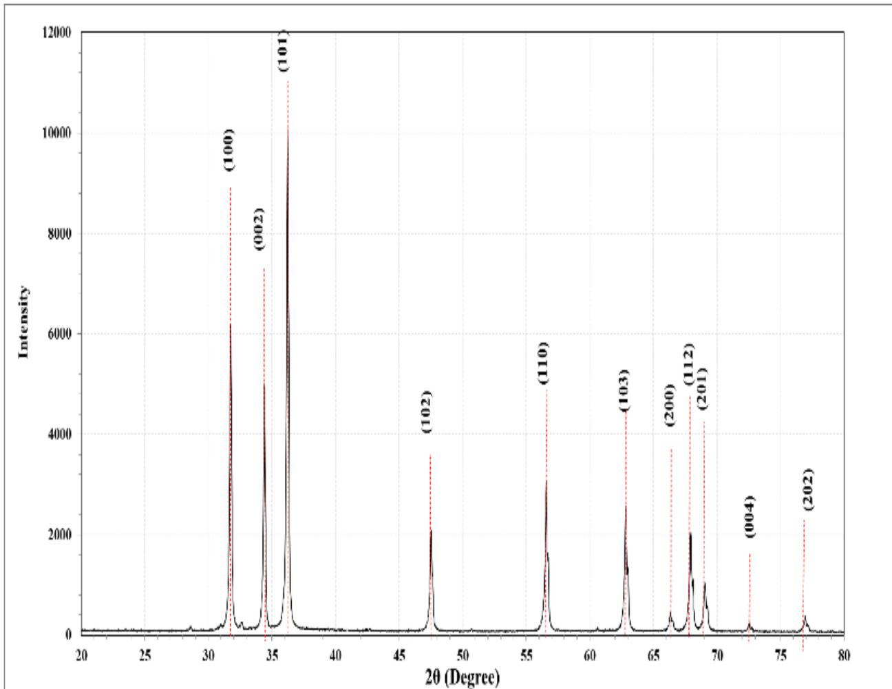
Figure 1. The X-ray diffraction diagram of ZnO powder
