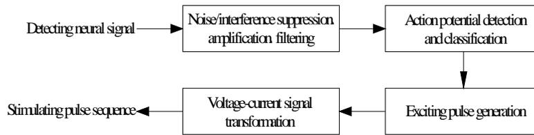
**Figure 3.** Flow chart of microelectronics nerve bridge data processing
