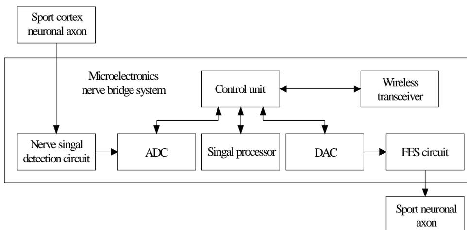
Figure 2. Block diagram of microelectronics nerve bridge system
