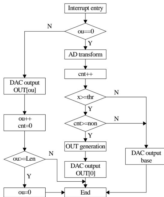
Figure 8. Flow chart of algorithm hardware program
