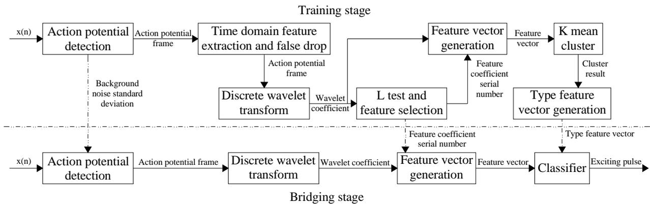
**Figure 4.** Data processing flow of training stage and bridging stage
