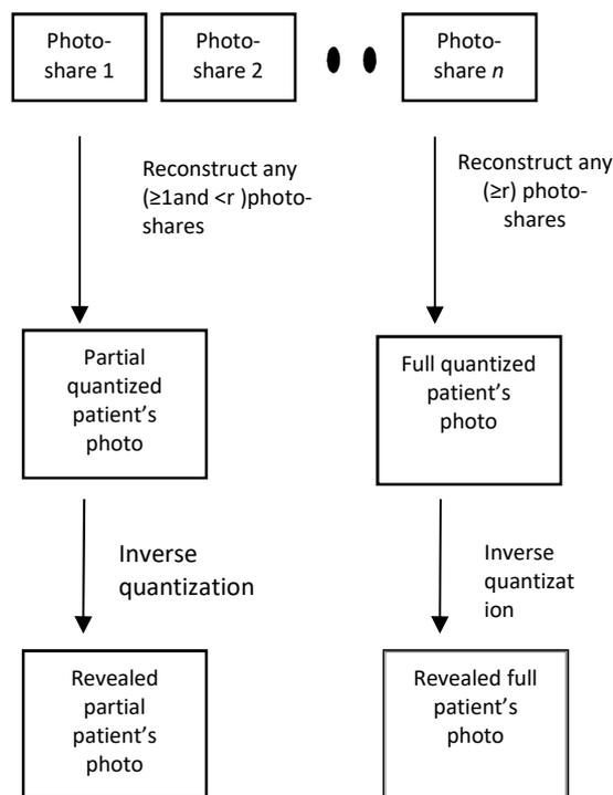
Figure 2. Flowchart of the decoding process
