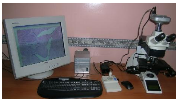
Figure 2. A CAS system. This system consists of software, a digital camera, microscope, and monitor. The stage of microscopy is controlled by the software, which also records data during the stereological procedures.
