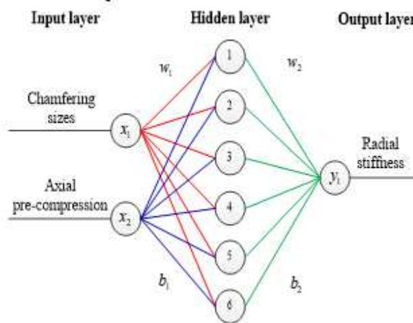
Figure 2. Structure of BP neural network model
