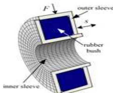
**Figure 6.** Finite element model of rubber bush inside dynamic vibration absorber
