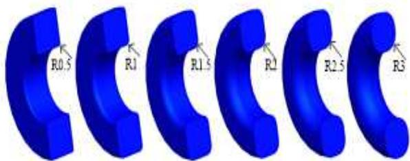
Figure 7. Rubber bushes of different chamfering sizes
