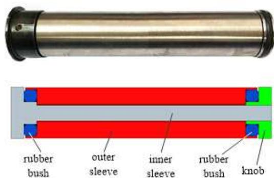
**Figure 1.** Structure of the dynamic vibration absorber
