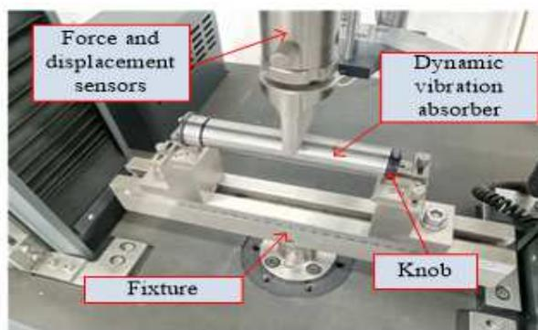
**Figure 4.** Test of radial stiffness under different axial pre-compressions
