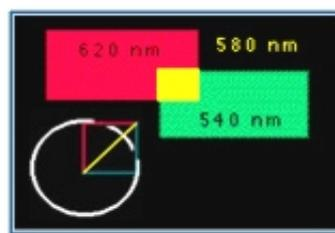
Figure 2. Vector superposition; notice that the normalized yellow vector is a precise metamer for yellow at 580 nm.
